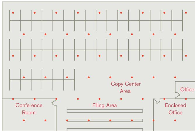
Quiet Technology™ sound masking attaches to furniture, so efficient coverage results from targeting only those areas of the space that require sound masking.
